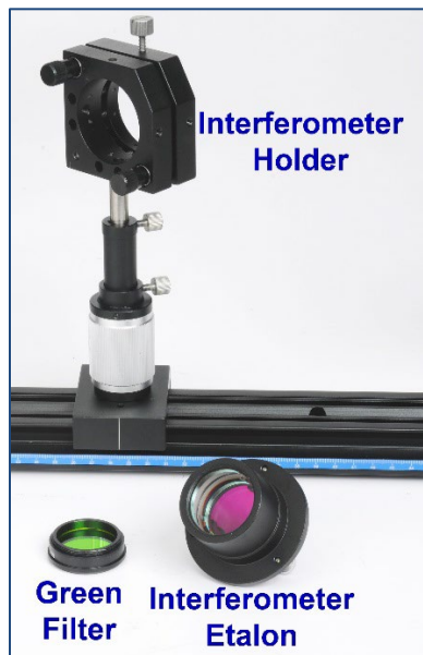
Figure 14: Filter and Interferometer
